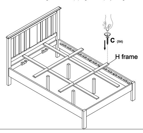
STEP 4: Attach 7 onto 3 using the screws (C), tighten it up by using an screwdriver.
